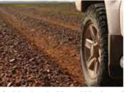
something you can always feel by hand either. Chipping of the tyres is minimised by lower speeds and lower pressures to improve the tyres resistance to objects and also heat build up. Higher pressures will be required when carrying heavy loads.
