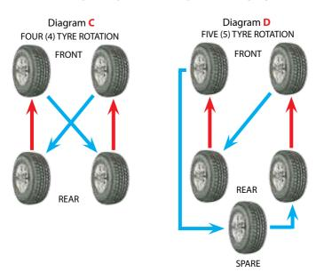
FOUR (4) & FIVE (5) TYRE ROTATION PATTERN FOR VEHICLES WITH DIFFERENT SIZES FOR FRONT & REAR AND DIRECTIONAL PATTERN TYRES
